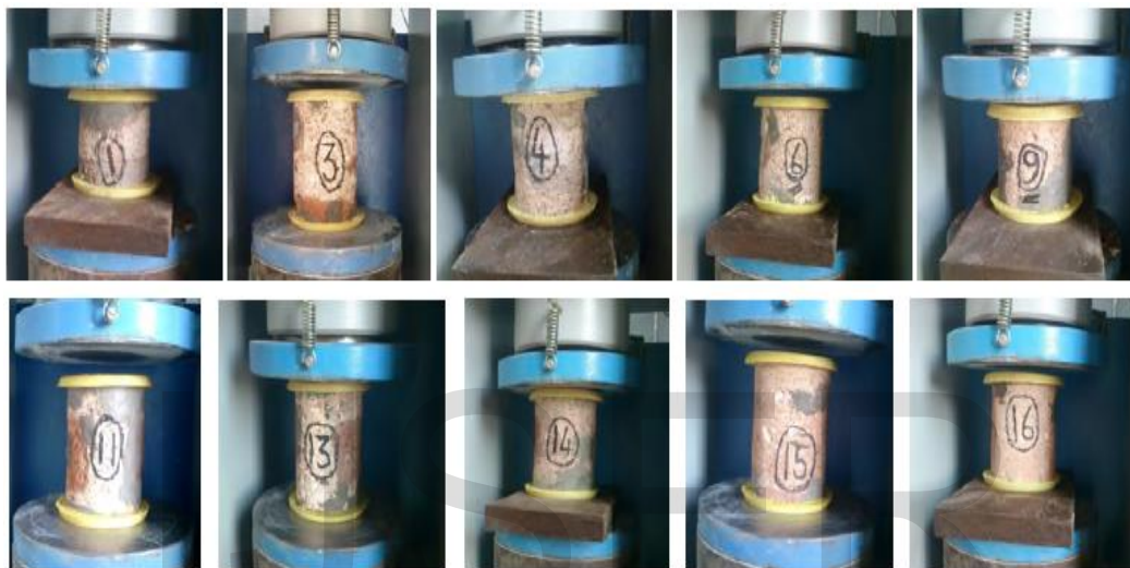
Fig. 5 Compression testing in laboratory of core samples [12]
